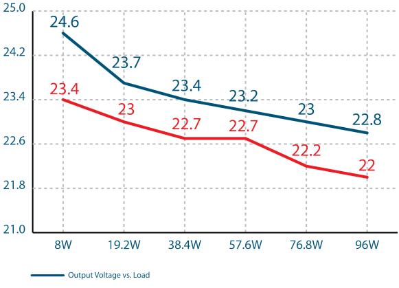
Output Voltage With a Typical TRIAC Dimmer (on Max)
